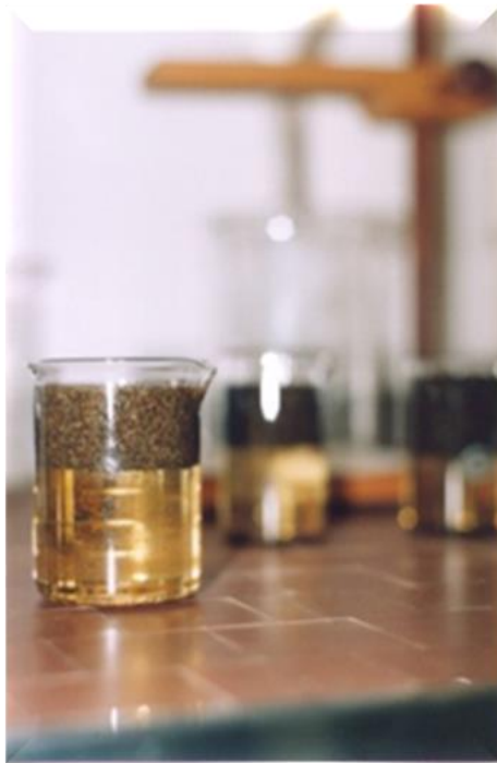
Mineral separation using an heavy liquid (2.89 g/cm 3 )
