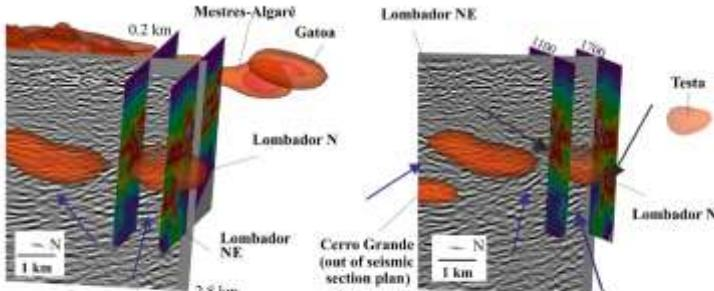
Figure 9. Correlation between 3D seismic cube, TEM reprocessed data over location in Fig. 4c and high-density anomalies of Lombador North gravity anomaly. The figure shows two seismic sections: one from Mestres-Algarv to Gatos, and another from Lombador NE to Testa. Both sections show geological features like the Cerro Grande (out of seismic section plan) and Lombador N. Arrows point to seismic reflections (blue) and high-conductivity anomalies (black) associated with Lombador N gravity anomaly.
