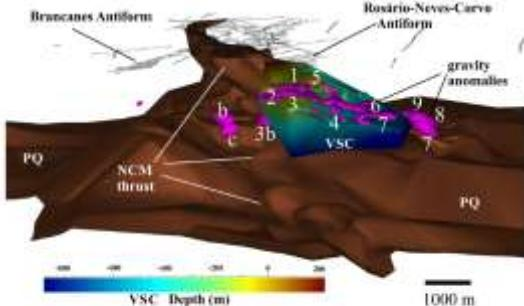
Figure 5. Gravity inversion results for the third series of runs compared with the surface of the top of PQ. It can be observed that high-density anomalies produced by the inversion and known deposits (pink bodies) are placed in the 3D model close to the TLYNC and the Neves-Corvo main (NCM) thrust, as expected. Density of  $>3.7 \text{ g/cm}^3$  are shown. The geological contours and faults of Figure 1b are overlain. Some gravity anomalies have been labeled.
