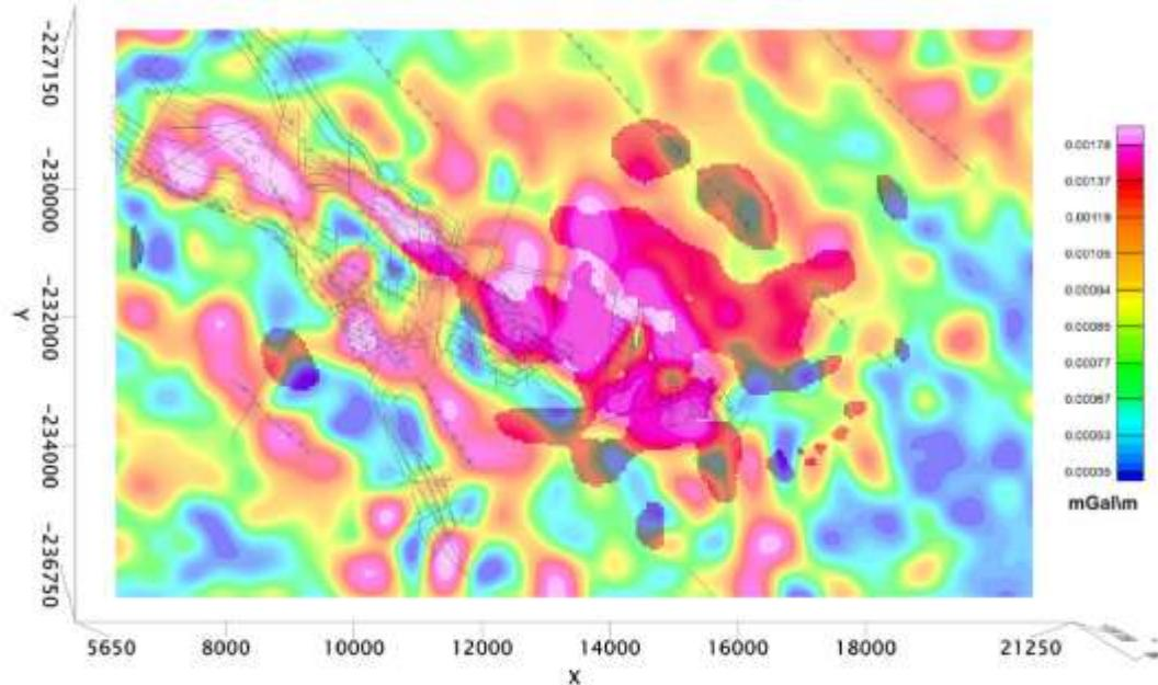
Figure 10. Results for the third run of the gravimetric inversion ( $d > 3.5 \text{ g/cm}^3$ ) overlaid by the analytical signal of the residual Bouguer anomaly map shown in Figure 2b. Geological contours of Figure 1b are also superimposed.
